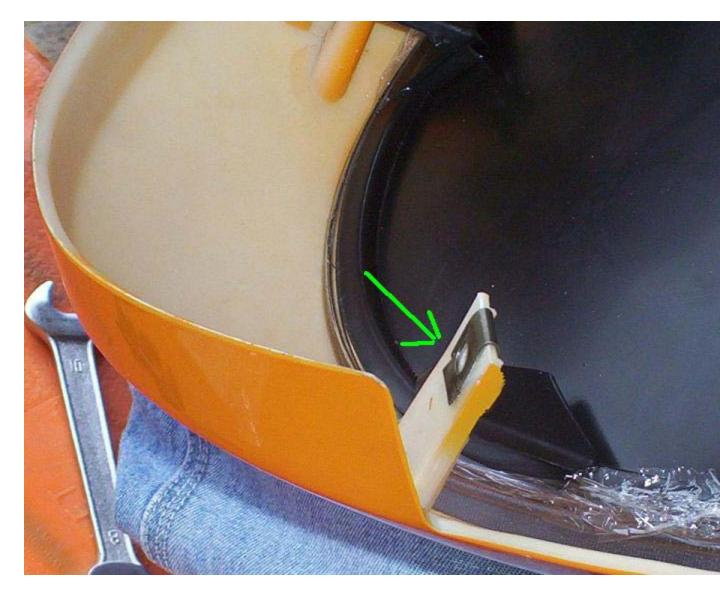
7A) Plug in the headlights, (the white connections,) before attaching the fairing. PLEASE NOTE: The headlights will not work until the scooter is started.
