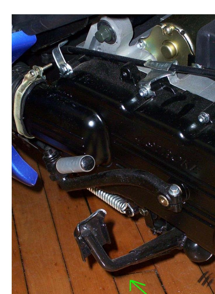
3A) Remove the black plastic spacer by the brakes, (see photo below.)
