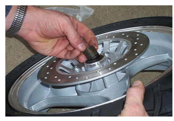
3C) You will need to slide the axel rod all the way through both sides and securely attach it.
