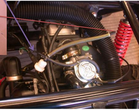
Connect the fuel line with the fuel tank
