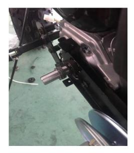
C) Put on the inside piece of the front clutch and check the alignment (adjust the washer to make it straight)
