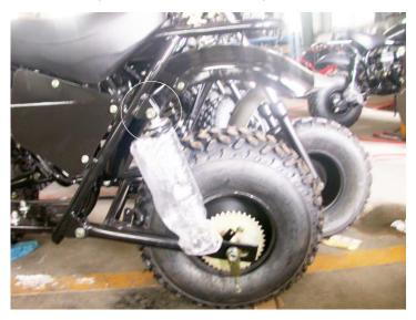
2. Install the front fender: Install the front fender between the fork using bolt M6x16 and nut M6 (The fender is to install in the middle of the fork, the space to left and right side of the fork should be the same.)
