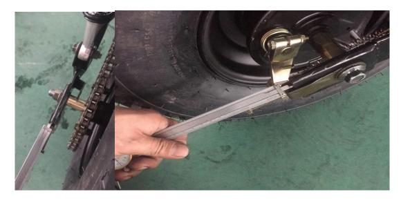
C) Tighten the adjuster bolt
