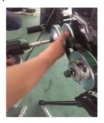
F) Tighten the M16x1.5self-locking nut on the driven pulley with torque 75-83Nm
