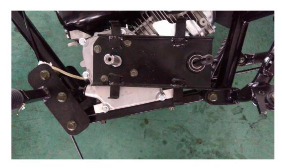
7. Install the flat key and 10 teeth sprocket (note: if your mini bike comes with pre-assembled engine, you may skip this step)
