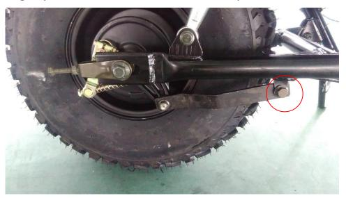
B) Adjust the chain adjuster bolt to chain has up to 3/8 inch tension space in vertical direction. The adjustment on left and right side of the chain adjuster should be equal.
