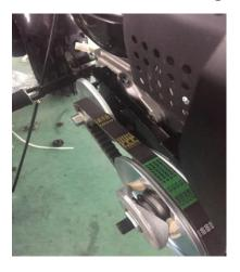
E) Install the front clutch bushing, front clutch cover. Tighten the M8x55 bolt with torque 22-29Nm
