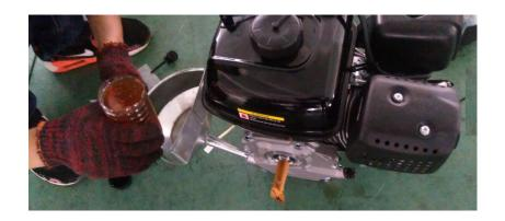
5. Install the clutch jackshaft plate 58200-L: (note: if your mini bike comes with pre-assembled engine, you may skip this step), attach the jackshaft 58200-L on the engine using M8x16 bolt, please do not tighten all the bolts at this step.
