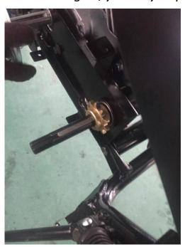
8. Install the drive chain: (note: if your mini bike comes with pre-assembled engine, you may skip this step) open the master link, put the chain around the sprockets, lock the master link (Caution: the direction of the master link opening is opposite to the chain forward movement direction)
