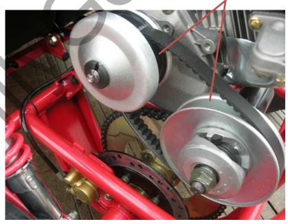
Caution: The two sides of CVT belt are not same, <u>one side is plane</u> <u>and other side is inclined</u>. The plain side and inclined side of CVT belt must match the plain and camber surface of clutch and pulley.
