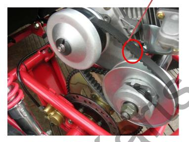
If it's determined that both plain surfaces of clutch and pulley are not aligned, the adjustment is necessary: loosen the <u>4 bolts</u> which fix the engine, and move the engine with front clutch to align with the driven pulley, and then fix the bolts. Measure again before driving to ensure the planeness of two interior surfaces is in the tolerance of  $\pm$  2mm.
