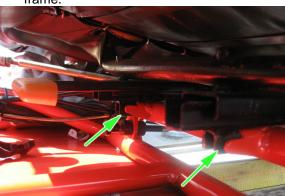
b. Slide the seat forward using the adjusting lever. This will make mounting the fasteners in the rear of the seat more accessible. Fasten rear seat bracket to the frame with the nuts and bolts.
